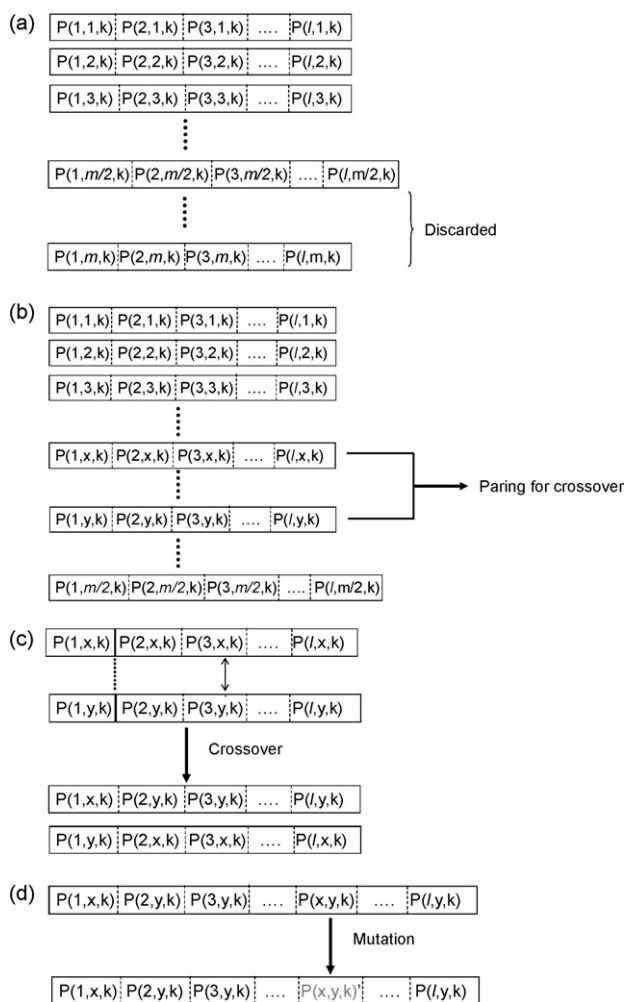
Fig. 3. The sub-processes of the genetic algorithm as gene extinction (a), pairing for crossover (b), crossover (c), and mutation (d).
